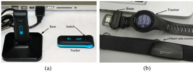
Fig. 1. System components: (a) Fitbit: trackers (one cradled on the base), the base (arrow indicated), and a user laptop. The arrow pointing to the tracker shows the switch button, allowing the user to display various fitness data. (b) Garmin: trackers (the watch), the base (arrow indicated), and a user laptop.
